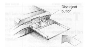
The disc clicks into place when it is fully inserted.
