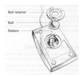
Wipe the ball with the clean, dry cloth. Do not use a cloth which may leave lint, and do not use cleaning liquid on the ball.
