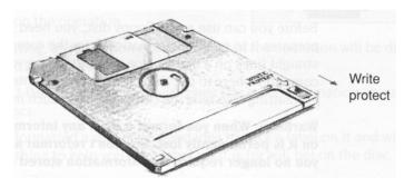
Remove write-protection by moving the tab back again.
