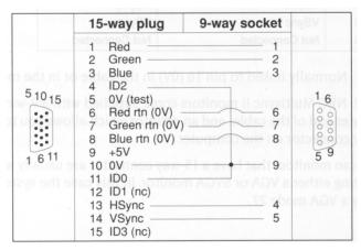
Most Multiscan monitors are now being designed to be VGA-compatible and will work satisfactorily when driven with separate horizontal and vertical sync signals.
