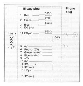
Note: HSync (pin 13) linked back into ID0 (pin 11) tells the computer that Composite sync (CSync) is required rather than VSync on pin 14 and that only modes compatible with a TV standard monitor can be displayed.
