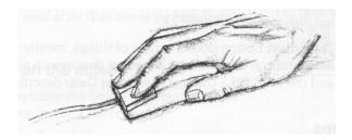
Move the mouse around and watch the pointer move around the screen. If you run out of space to move the mouse, lift it up and put it down again in a more convenient position. While the mouse is lifted, the pointer will not move, and when you put it down again you can carry on where you left off.
