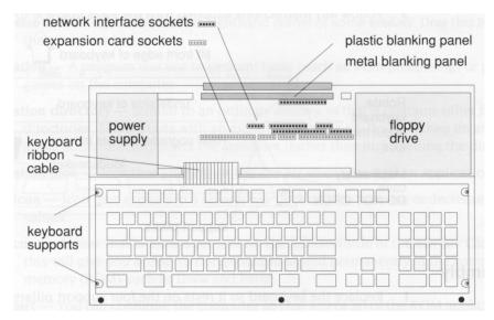
If you ever remove an internal expansion card, make sure you replace the two blanking panels before you use the computer again.
