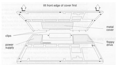
4 When the clips are free from their slots, lift the top plastic cover right off.
